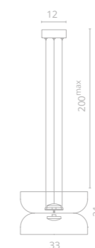
2 5246/33 SP-10 ø33 | 121 | 200 max 1x10W LED 500Lm 4000K CRI≥80 Bulb incl.
